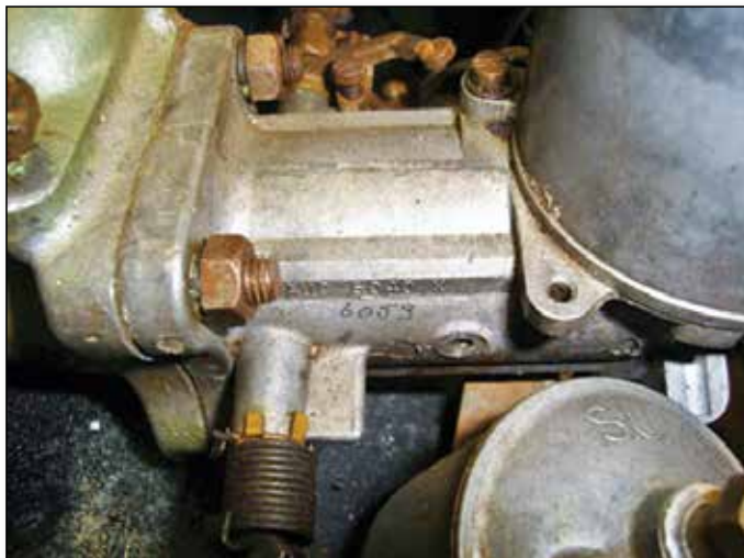
Both 100M carburetors have special embossed and engraved numbers on their sides.
