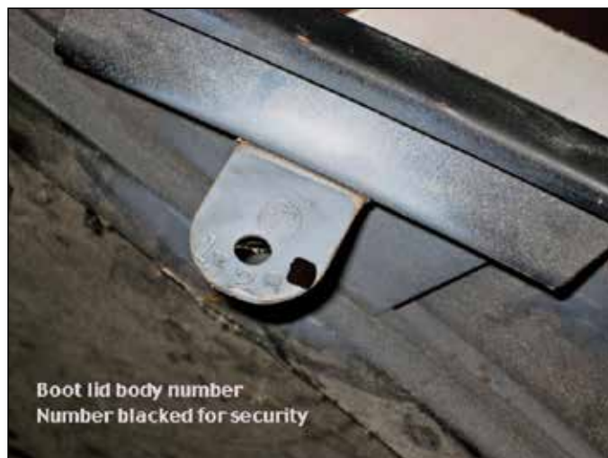
Each 100 has a boot lid bracket with the body number stamped in it.
