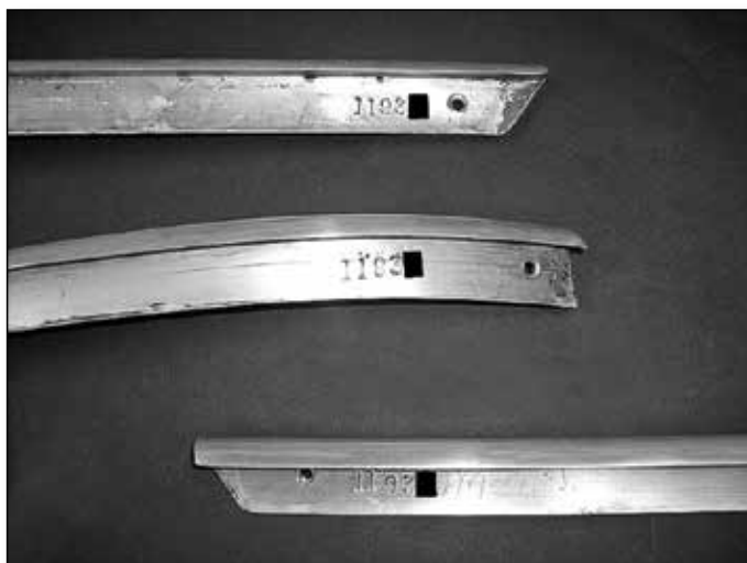
Cockpit surrounds were hand fitted and numbered. Note that this is how the cockpit surrounds should be photographed for registration: all in one photo.
