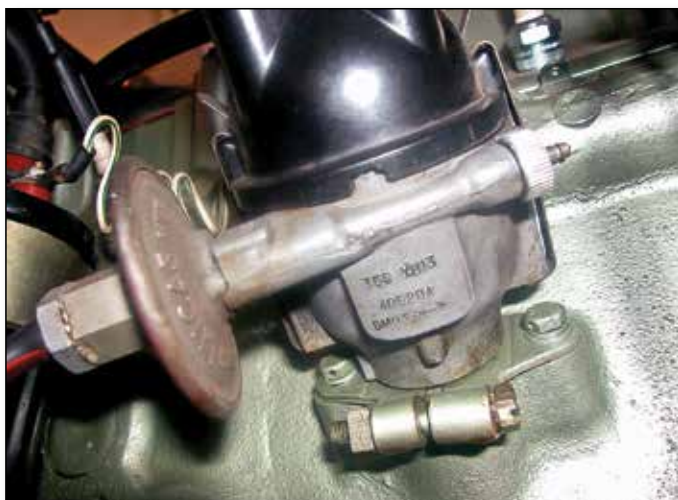
The factory-built 100Ms had special distributors, model number 40522 on early examples and 40520 on all later ones.
